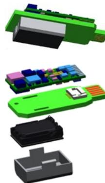
The speaker enclosure is removed by unclipping (it is held by 2 clips).
